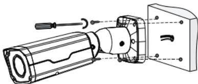
Lead tapping screws through the guide holes in the base and fix them to the wall by using a screwdriver.
