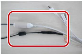
3. Protect other cables using insulating tapes.
