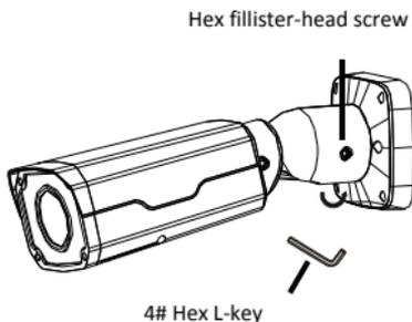
5. Mount your camera onto the wall and connect all cables.
