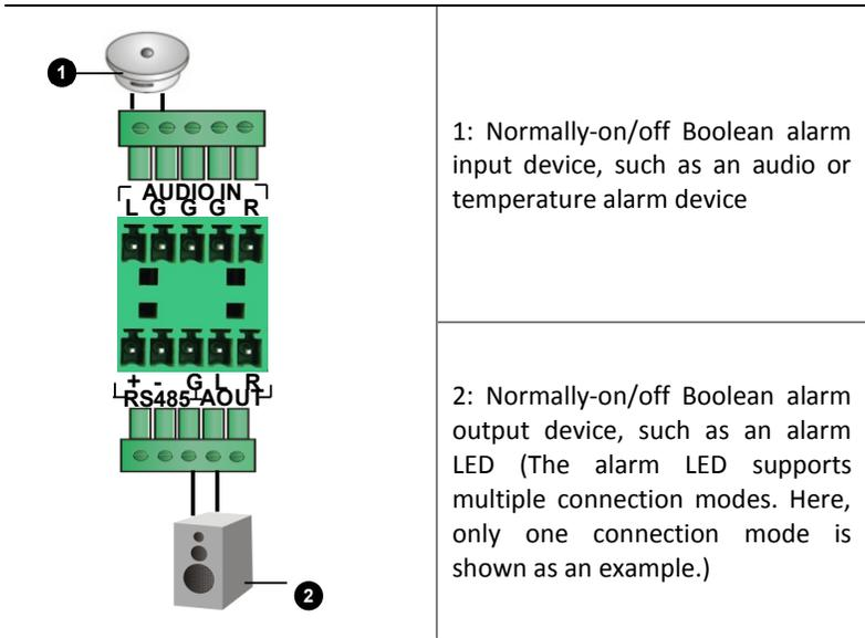
1: Normally-on/off Boolean alarm input device, such as an audio or temperature alarm device
